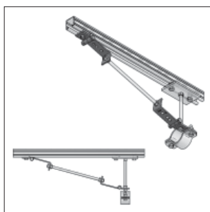
Joint angle with bracing
